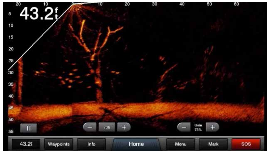
Forward Facing Sonar allows anglers to have a two-dimensional live view of everything going on under the water around their boat. Notice the fish being picked up by the Garmin Livescope.
